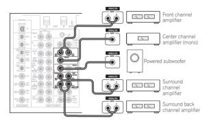
• You can use the additional amplifier on the surround back channel pre-outs for a single speaker as well. In this case plug the amplifier into the left (**L (Single)**) terminal only.
